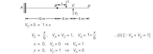
CD: When unit load is between C and D (At x from C)
